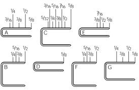
Available Crown Widths 3/16", 3/8", 1/2". 22 Gauge Staples. 5/32" - 5/8" Lengths. Capacity 110-185.
